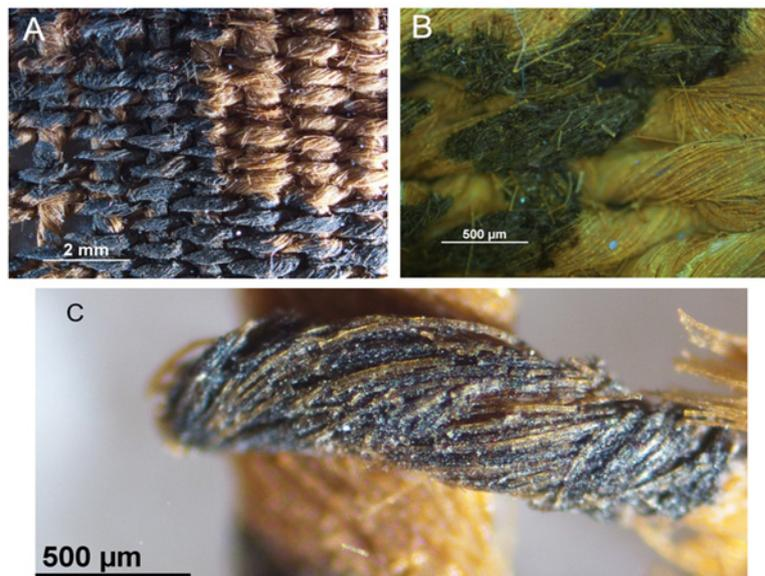
Fig. 4. UV-VIS microscope images of (a, b, c) textile samples painted with carbon charcoal. The images show clearly the mask and deposition of the particles on and in-between the fibre surfaces.
