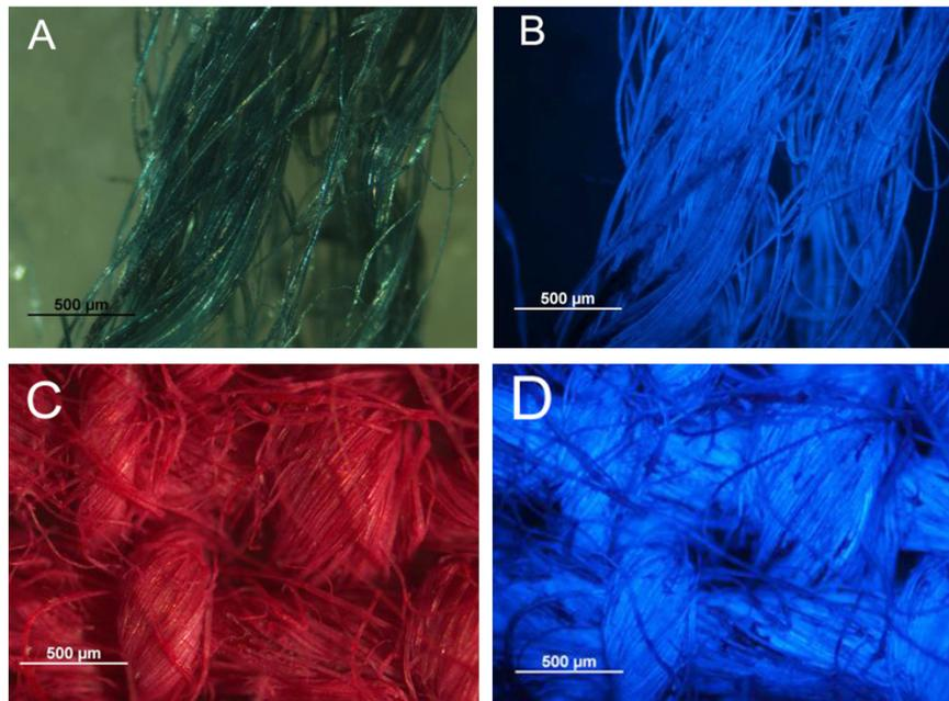
Fig. 3. UV-VIS microscope images of (a, b) fiber samples dyed with indigo dye, (c, d) Cochineal-dyed sample.
