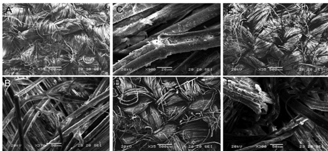
**Fig. 6.** SEM microphotographs of the dyed textile samples with (a, b) indigo, (c, d) madder, (e, f) cochineal, show that the dye molecules are small enough to penetrate into the fibres without changing the fibre morphology. Also show minor degradation of the linen fiber surface after thermal ageing as small scratches and longitudinal splitting.
