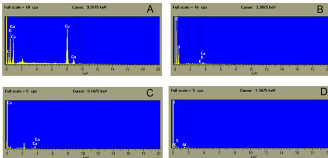
Fig. 7. EDX results of the experimental coloured textile fibres with (a) malachite, (b) black charcoal, (c) calcite and (d) madder.
