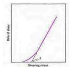
Fig.16. Flow curves of plastic flow
