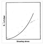
Fig.15. Flow curves of pseudo-plastic flow
