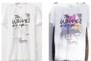
Before UV irradiation After UV irradiation Figure 4: Photochromic colorant effect
