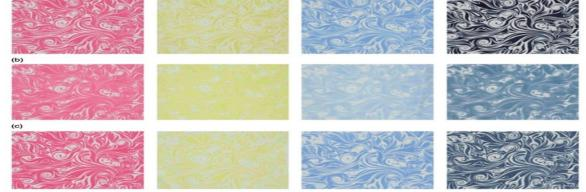
Figure 9. Fine pattern qualities of the printed silk satin using TDG, XG, and SA as thickeners at the same concentration of 3 wt % with different reactive dyes.
