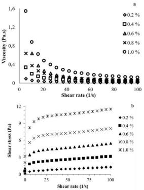
Figure 1 shows the viscosity and flow behaviour characteristics in relation to the shear rate at various RSG solution concentrations. Shear rate vs viscosity as seen on the surface, and shear rate versus shear stress.
