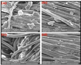
Figure 2 SEM images of treated cotton fabric with RTV silicon /chitosan using different concentration
