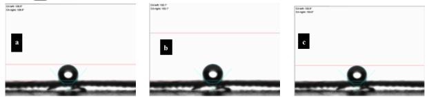
Fig.2. Static water contact angles of the treated polyester fabric.
