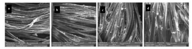
**Fig.1.** SEM images of treated polyester fabrics with  $ZnO(\underline{a},\underline{b})$ . images of treated cotton fabrics with silicone rubber ( $\underline{c},\underline{d}$ )
