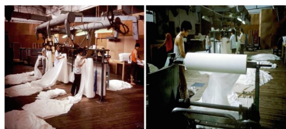
Fig. 6. Quality control of pure white silk fabrics
