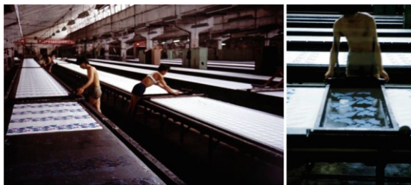
Fig.7. Printing of silk fabrics
