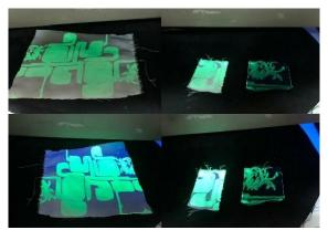
Fig.3. Images of photochromic dyes on the surfaces of polyester fabric that is treated with silicone rubber polymer and TiO2 NPs.
