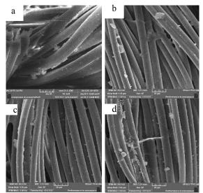
Fig.1. SEM images of the treated polyester fabric withsilicone rubber and TiO<sub>2</sub>NPs (3%)
