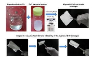
Fig. 5. Photographic representation of the preparation of alginate hydrogel/zinc oxide nanoparticle (n Zn O) composite bandages.
