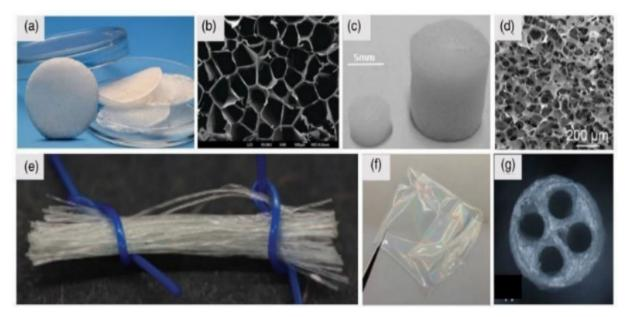
Fig. 8. Type I collagen-based collagen sponge discs (Sponge Col) in (a) and (b) scanning electron microscopy (SEM) images of the porous network structure. (c) Scaffolds of various sizes, and (d) an SEM view of a collagen scaffold made from jellyfish. (e) A group of type I collagen fibers that were extruded. (f) A collagen-type I translucent film. Neural conduit is made of several channels of type I collagen9. [73].
