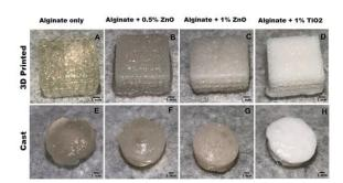
Fig. 4. (A–D) depict 3D-printed lattice structures. (E–H) portray manually casted structures. The scale bar in all images depicts 1 mm.
