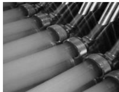
(Fig. 2) Extrusion of acrylic fibers from the spinneret. (Source: Courtesy of Aksa, a member of AKKOK Group of Companies, Turkey.)
