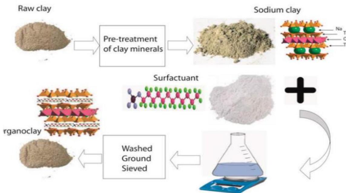
Figure 21: Preparation of organoclay
