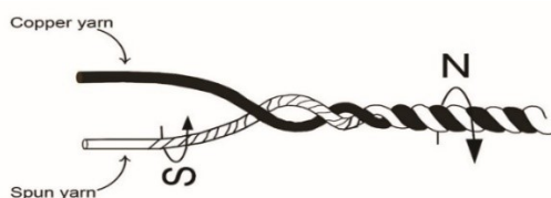
Figure 14: Plied yarn with copper as a component
