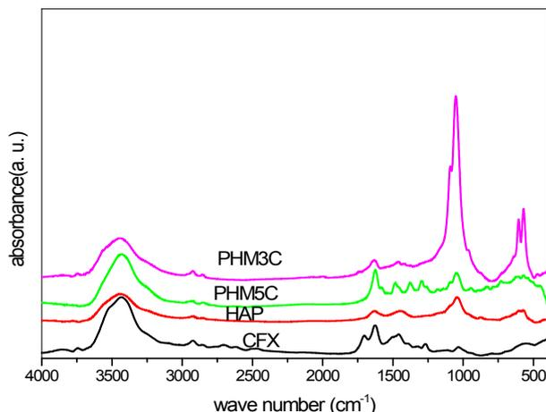
Fig. 3. FTIR spectra of pure ciprofloxacin (CFX), pure HAp and porous hydroxyapatite (HAP-10) /MWCNTs loaded with ciprofloxacin at various MWCNTs ratios (PHM0.5C and PHM3C).
