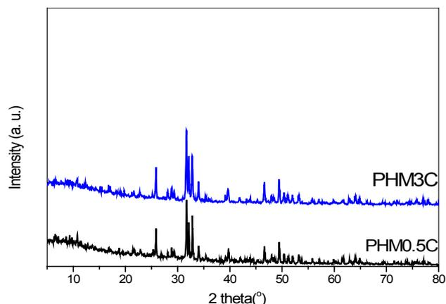
Fig. 5. X-ray spectra of porous hydroxyapatite (HAP-10)/MWCNTs loaded with ciprofloxacin at various MWCNTs ratios (PHM0.5C and PHM3C).
